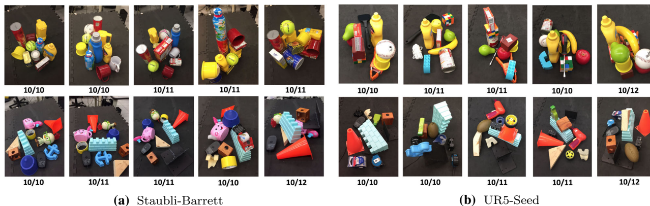
Fig. 5 Results for a few cluttered scenes used for real-world experiments for a Staubli-Barrett and b UR5-Seed. In each scene, there are 10 objects randomly and densely placed on the table. Sometimes objects in the scene overlap with each other, as shown in the two right-most scenes in each row for each robot. We report # successful grasps/#
