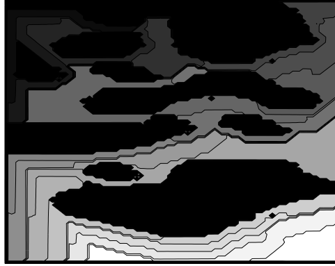
FIGURE H.9. A plot of linklength values from the start (upper - left corner) node where colored cells correspond to link lengths of paths defined by the depth-first search. The lighter the cell the greater the linklengths in the graph; black cells correspond to obstacles.
