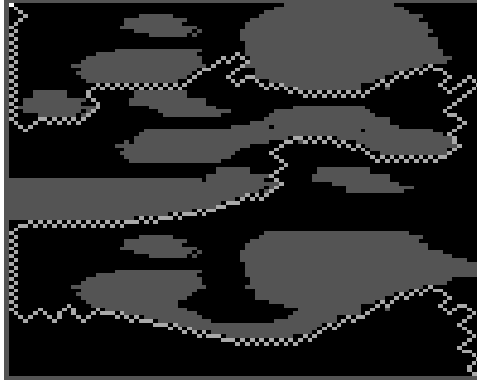
FIGURE H.8. White cells denote the path that was determined with depth-first search.
