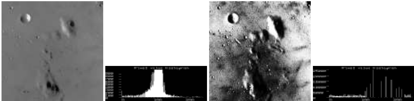
Figure 4: Histogram Equalization. Original image and histogram and equalized image and histogram. See http://www.dai.ed.ac.uk/HIPR2/histeq.htm .
