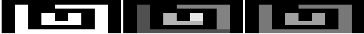
Figure 7: Blob coloring. Left: original binary image. Middle: blob color assignment after first pass. Right: Blob color assignment after merging colors.
