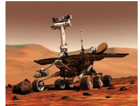
Mars rover Spirit used cameras for visual odometry
