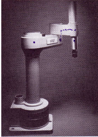
Figure 3: Adept 1 Scara Robot arm. This arm is in a R-R-P-R configuration. \theta_1, \theta_2, \theta_4 are the revolute joint angle variables and q_3 is the prismatic joint variable. The robot is pictured in the Home position in the frame diagram using the values of the joint variables listed in the table below.
