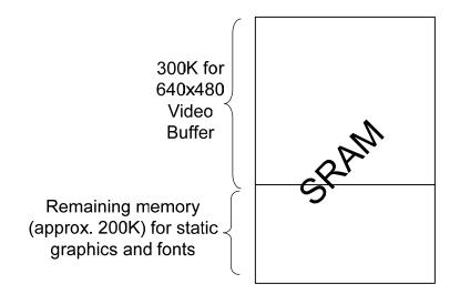
The figure above shows the memory map for the video buffer within the SRAM.
