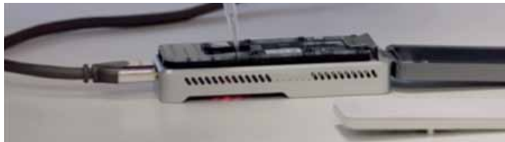
The MinION is four inches long, weighs 4 ounces, and gets power from a computer's USB port.
