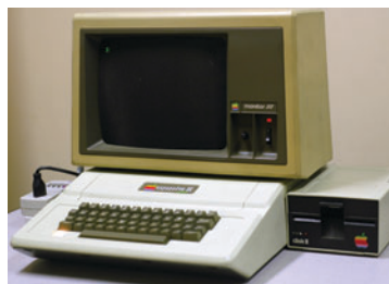
The original system: Apple II+; c.1982; Synertek 6502; LS TTL, 16K DRAMs, 1 MHz NMOS CPU; CPU: 4K transistors?; 22 Watts, 31 when disk spinning
