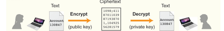
RSA is a single function where going one way is easy and one way is hard. It requires generating both a private and public key at the same time.
