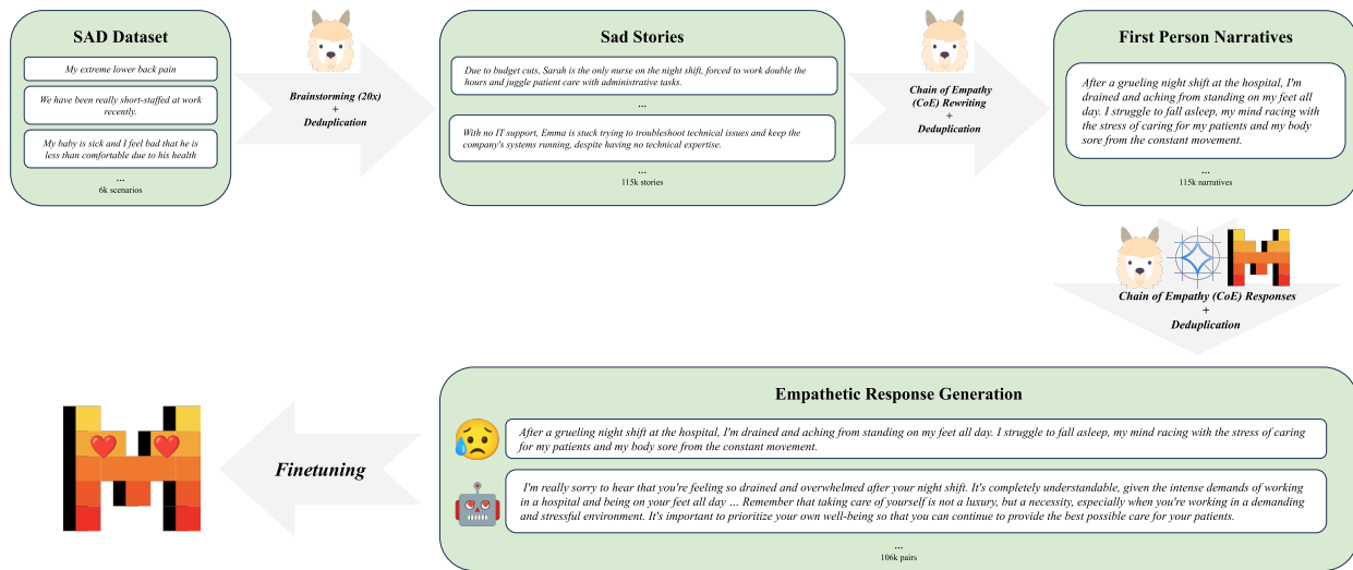
Figure 6.1: SYNTHEMPATHY Pipeline Overview. Stories are brainstormed from the SAD dataset [163], rewritten into first-person narratives using chain-of-empathy prompting, and used to generate psychotherapy-grounded empathetic responses. Each step includes deduplication, producing a dataset for fine-tuning LLMs in empathy.
