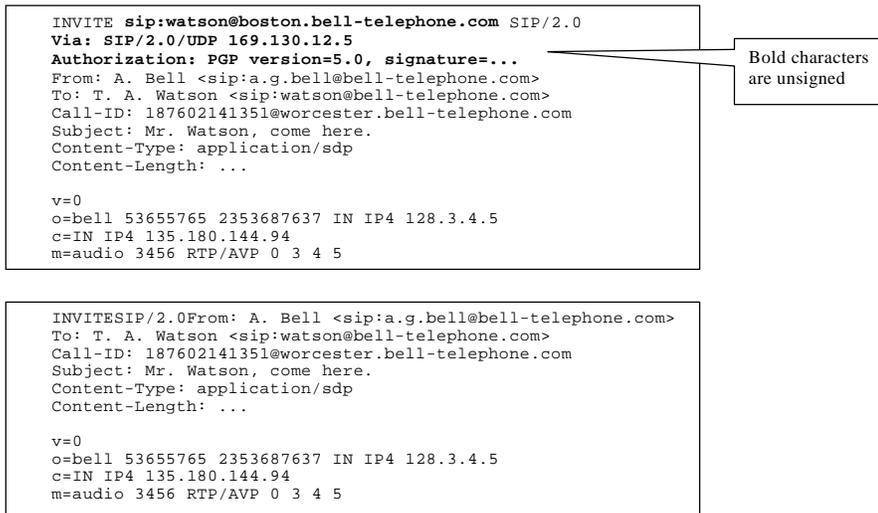
**Figure 29. Upper - the SIP request that is to be sent. Lower - the signed parts of the message**
