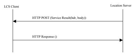
The following HTTP sequence diagram is used in the case of a General Error Message.
