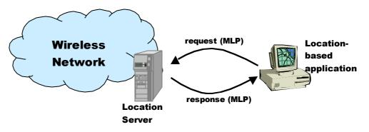
Possible realizations of a Location Server are the GMLC, which is the location server defined in GSM and UMTS, and the MPC, which is defined in ANSI standards. Since the location server should be seen as a logical entity, other implementations are possible.
