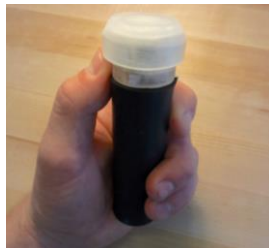
Fig 4. Prototype of Keppi , - tangible and portable self-reporting device for pain.
