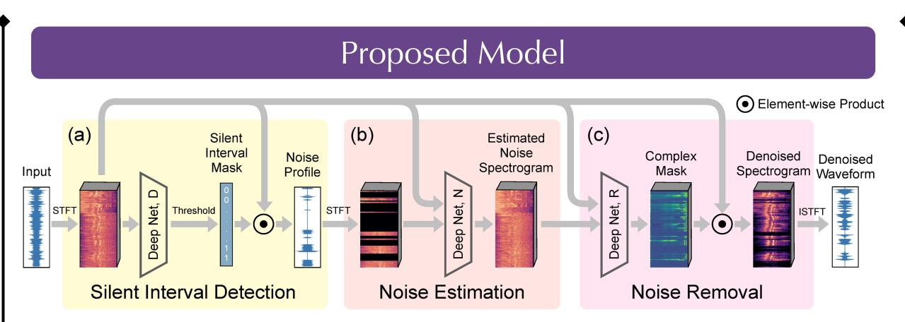
We propose a neural network that harnesses the time distribution of silent intervals for speech denoising. Our model has three components: (a) one that detects silent intervals over time, and outputs a noise profile observed from detected silent intervals; (b) another that estimates the full noise profile, and (c) yet another that cleans up the input signal.
