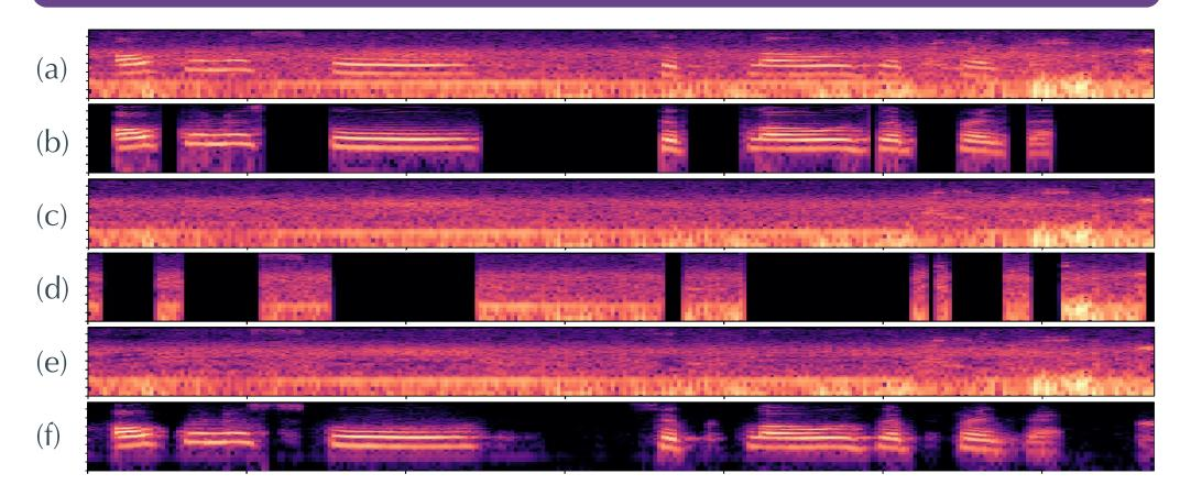
(a) The spectrogram of a noisy input signal, which is a superposition of a clean speech signal (b) and a noise (c). The black regions in (b) indicate ground-truth silent intervals. (d) The output of the silent interval detection component. (e) The estimated noise profile using subfigure (a) and (d) as the input to the noise estimation component. (f) The final denoised spectrogram output.
