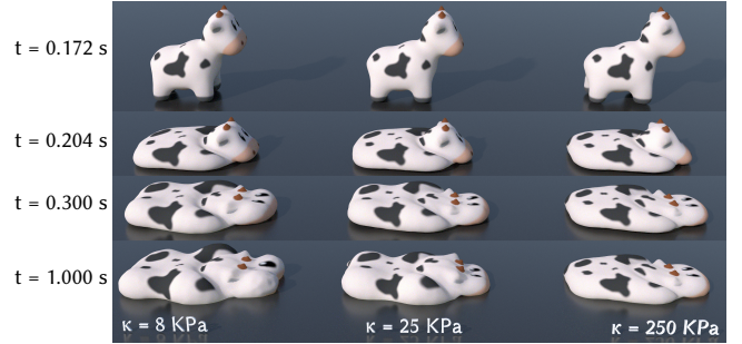
Fig. 8. Simulated cream with a wide range of bulk moduli ( \kappa ). Cream with a lower bulk modulus \kappa shrinks or dilates more easily during the simulation, and has a larger volume in the steady state.
