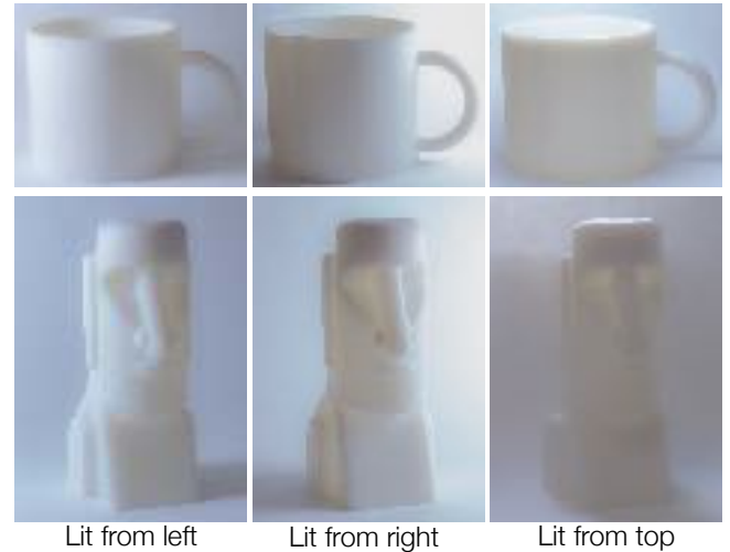
Figure 18. Under different extreme lighting, the embedded AirCode tags remain invisible. We capture these photos while moving a strong light source around the statue and the mug. The light source we use is a 45W photography light bulb at 6500K.
