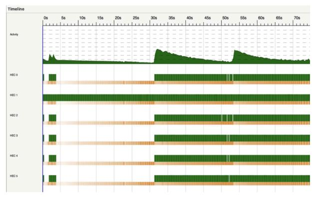
HEC 1 (main thread) shows consistent activity throughout execution, handling grid initialization, spark creation, and result collection. Other HECs (worker threads) show intermittent activity corresponding to spark execution from the work pool. During peak computation periods (30-55 seconds), all HECs display substantial green activity, confirming effective parallel work distribution.
