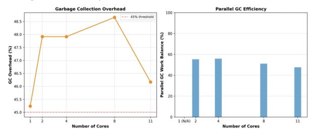
GC overhead remains stubbornly constant at 45-48% across all core counts. This is characteristic of functional implementations with high allocation rates. The parallel GC work balance of 47-56% indicates moderate efficiency - perfect balance (100%) is theoretically impossible due to generational GC design having inherent sequential phases.
