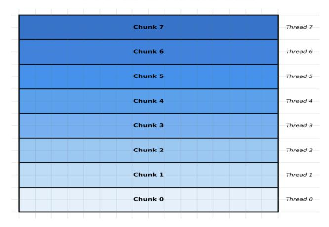
Each chunk processed independently in parallel Boundary cells can access original grid for neighbor information
