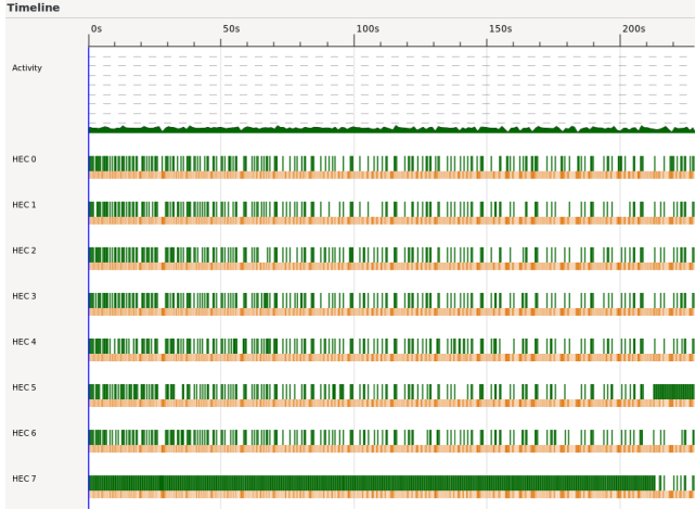
Figure 24: Threadscope chart for the non-overlapping batches in parallel method with eight cores
