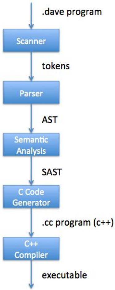
The architectural design of DAVE is demonstrated in the block diagram above. It is split into 4 major sections: Scanner (scanner.mll), Parser (parser.mly), Semantic Analysis (semanticAnalysis.ml), and C++ Code generator (compile.ml).
