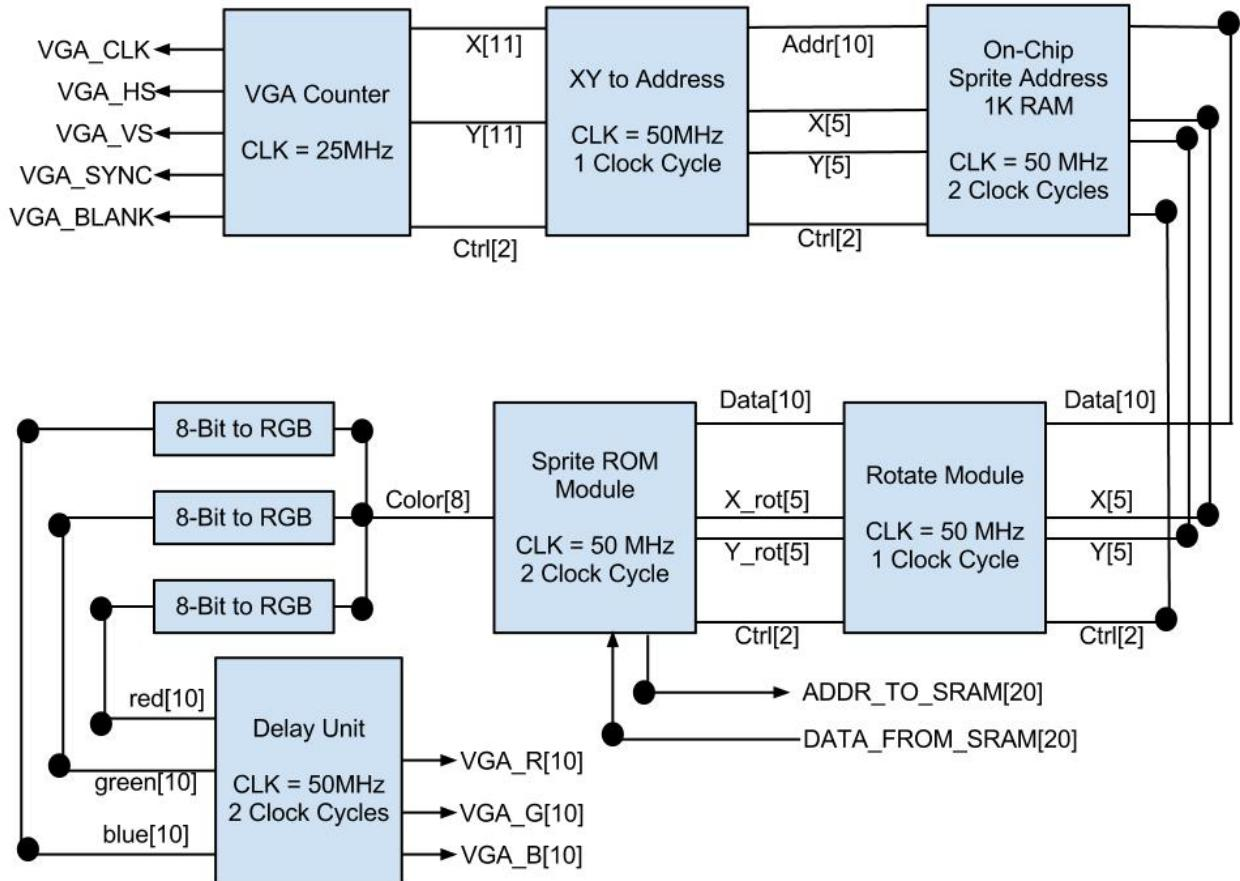
Note that all synchronization signals are passed through all blocks to ensure full system synchronization.
