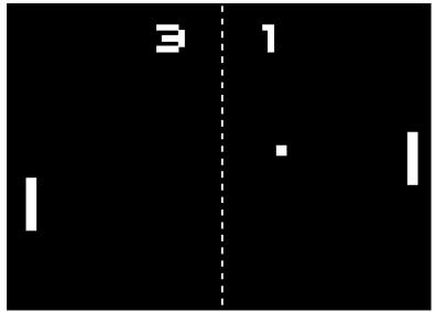
Our team decide to design a Ping-Pong video game. The rule is easy: hit the ball or loss. The game can be displayed on VGA and controlled by keyboard or mouse. Player can paly with AI or other one on same keyboard or different FPGA board through Ethernet.
