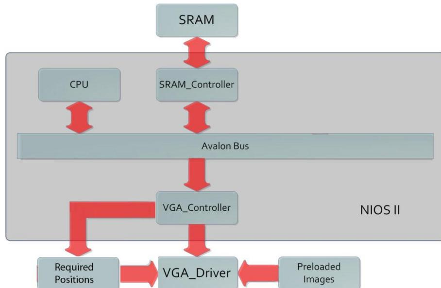
VGA display is to draw the game scenario, user interfaces and sprites in real-time. The data and instruction communications are completed via the Avalon bus. The VGA display function mainly contains 4 modules: VGA\_Controller, VGA\_Driver, Preloaded Images and Required Positions.
