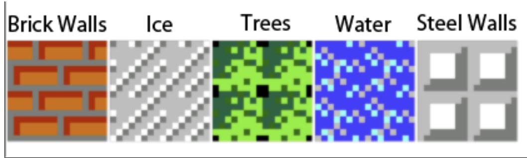
Static scenario could be constructed by simply replicating  $\frac{1}{4}$  of itself in order to reduce memory size. The VGA\_Driver only need the information of its position and type from RAM.
