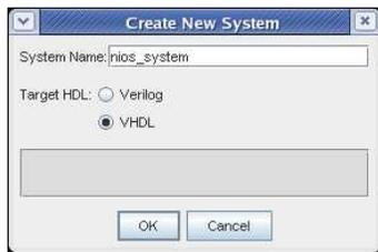
Figure 3: Naming a new system in SOPC Builder
