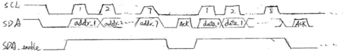
Figure 2. I<sup>2</sup>C Block and Timing Diagram
