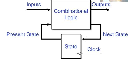
This is a *Mealy* FSM: outputs may depend directly on inputs.
