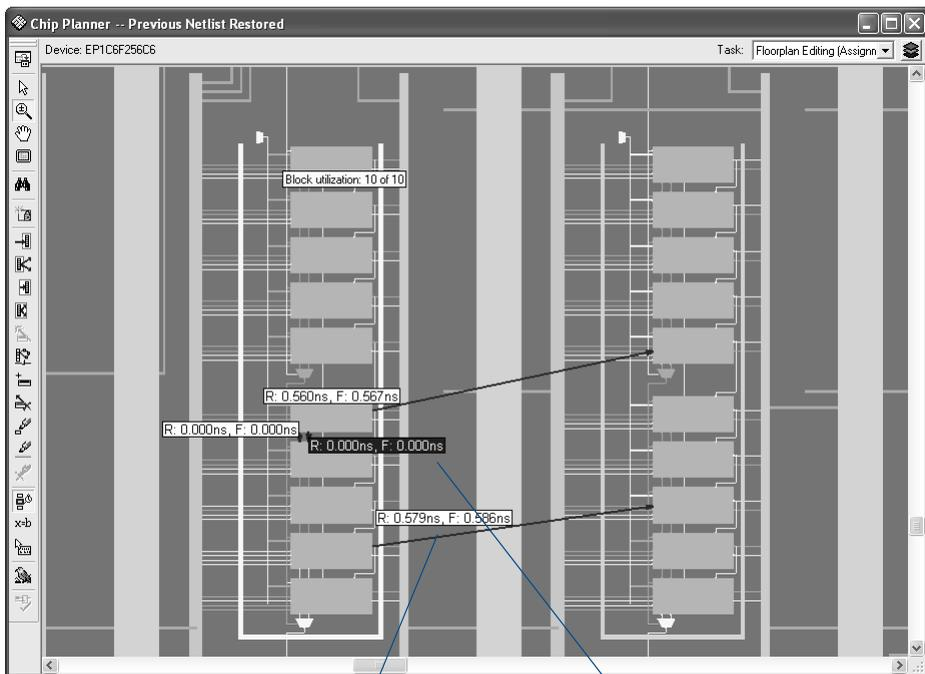
*Displays fan-in and fan-out connections of a selected resource*
