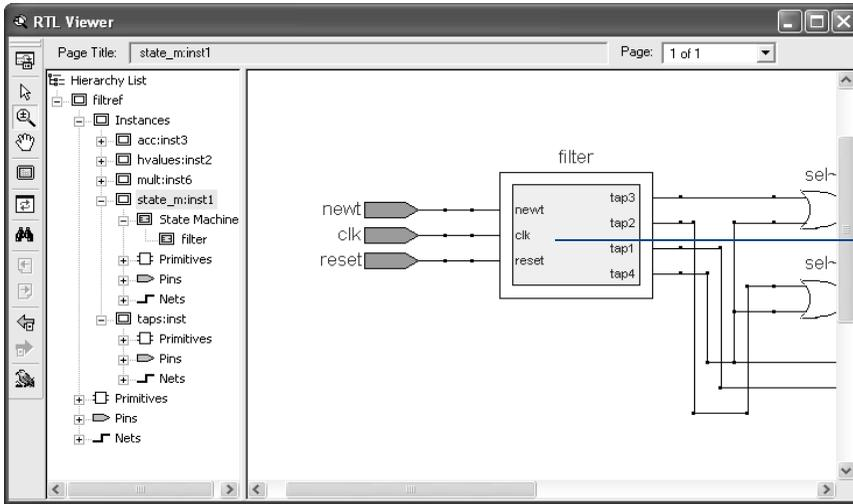
The State Machine Viewer includes a schematic view and a transition table (Figure 8).
