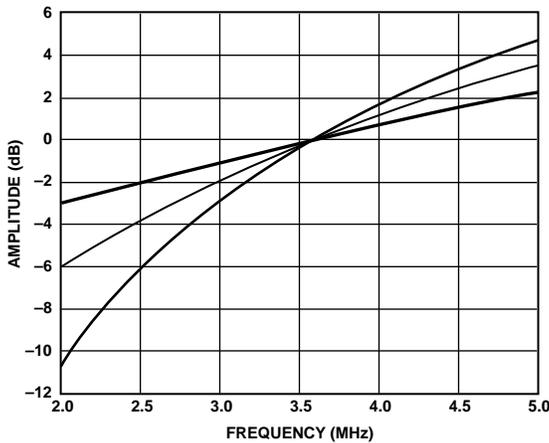
Figure 35. NTSC IF Compensation Filter Responses
