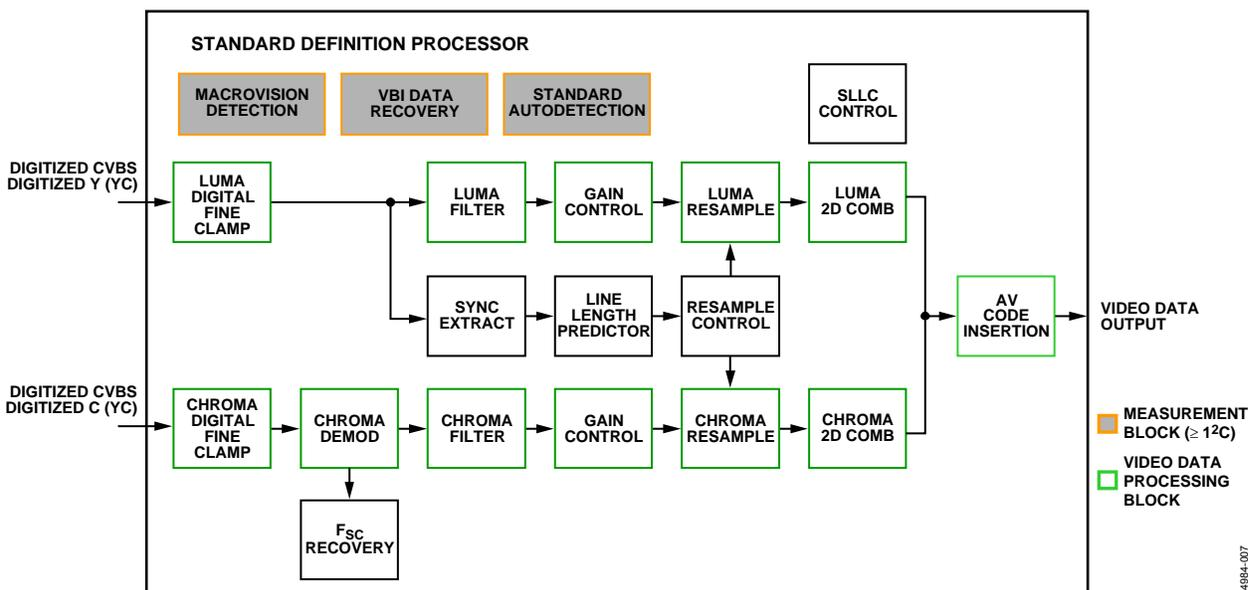
Figure 7. Block Diagram of the Standard Definition Processor
