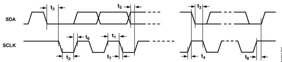
Figure 2. I<sup>2</sup>C Timing
