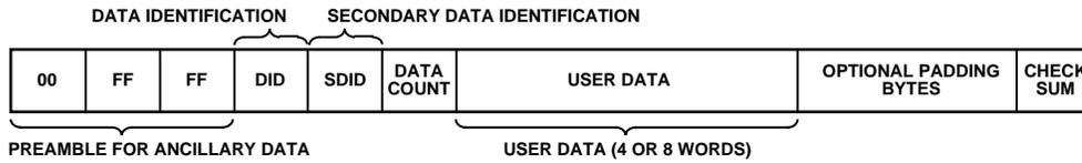
Figure 34. Gemstar and CCAP Embedded Data Packet (Generic)
