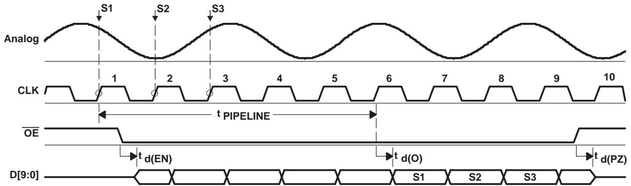
**Figure 2. Input Timing**
