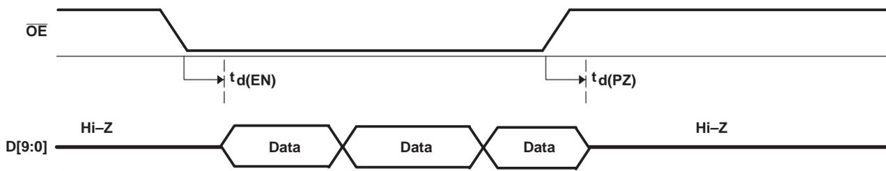
**Figure 3. Output Timing**
