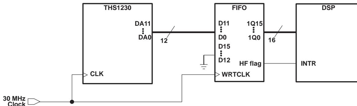
Figure 20. FIFO Connection
