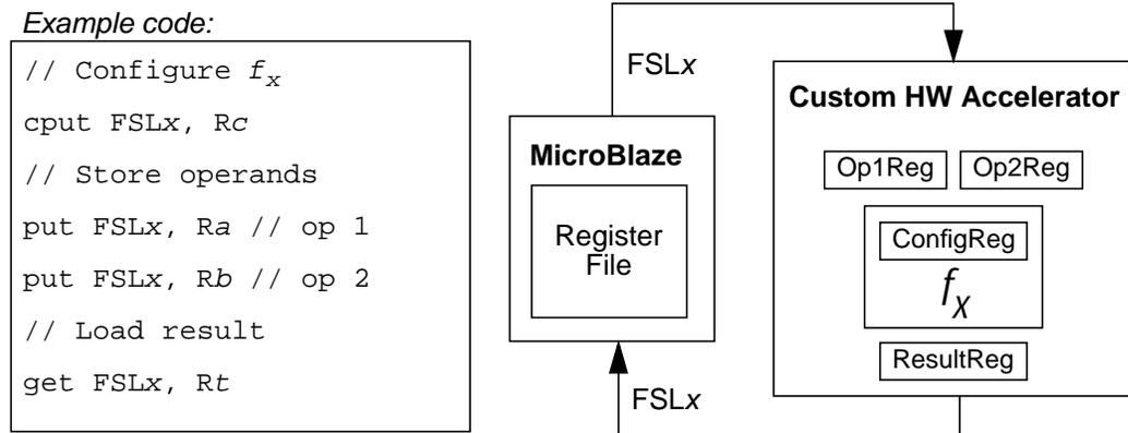
Figure 1-13: FSL used with HW accelerated function  $f_x$
