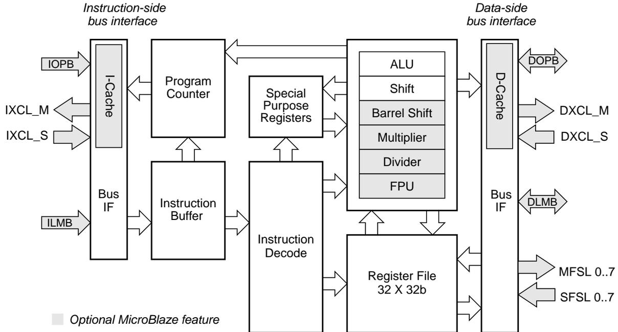
Figure 2-1: MicroBlaze Core Block Diagram
