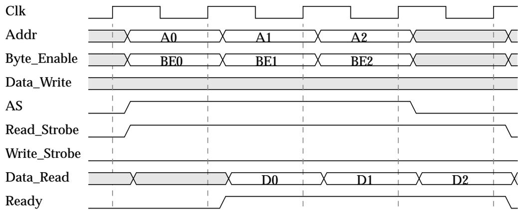
Figure 2-5: LMB Single Cycle Back-to-Back Read Operation
