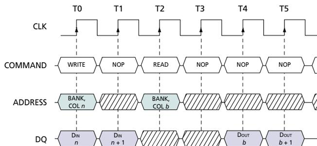
NOTE: The WRITE command may be to any bank, and the READ command may be to any bank. DQM is LOW. CAS latency = 2 for illustration.
