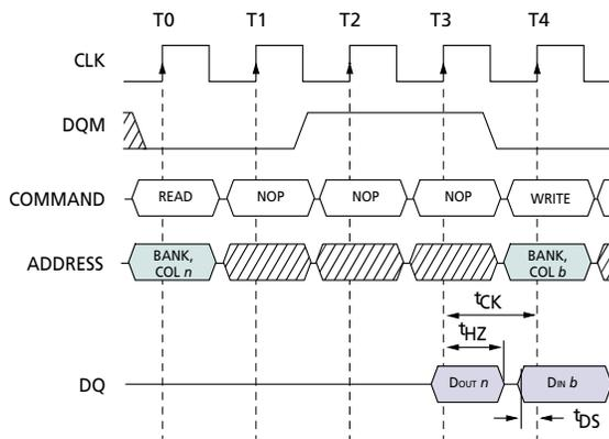
**NOTE:** A CAS latency of three is used for illustration. The READ command may be to any bank, and the WRITE command may be to any bank. If a burst of one is used, then DQM is not required.
