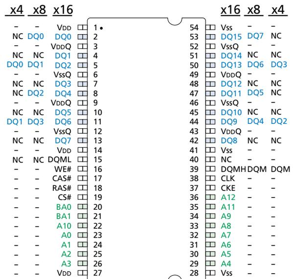
**Note:** The # symbol indicates signal is active LOW. A dash (-) indicates x8 and x4 pin function is same as x16 pin function.
