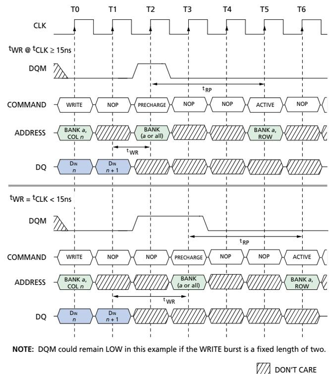
NOTE: DQM could remain LOW in this example if the WRITE burst is a fixed length of two.
