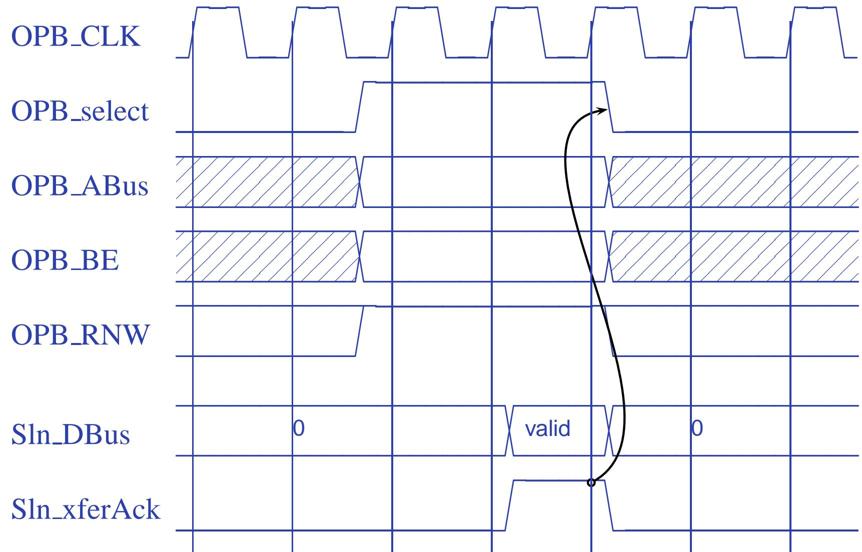
OPB signals arrive late; DBus and xferAck needed early.
