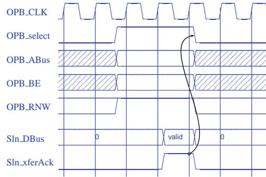
OPB signals arrive late; DBus and xferAck needed early.
