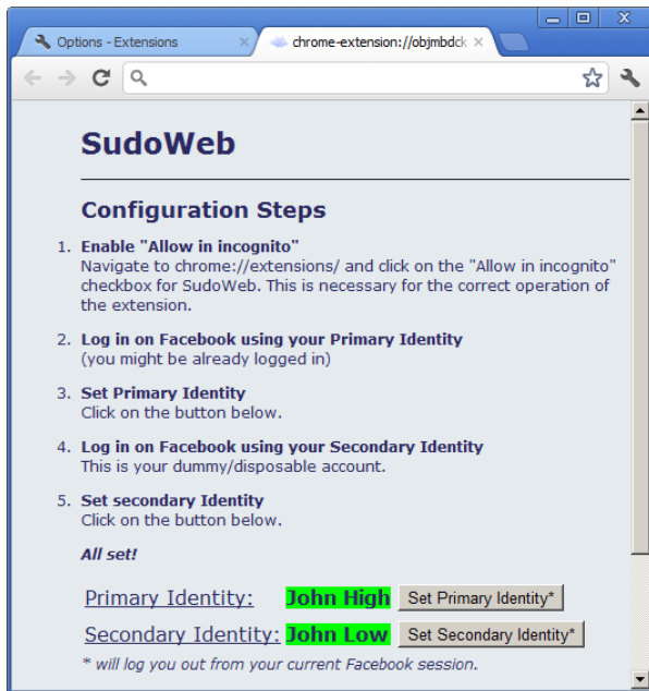
Fig. 6 Screenshot of the configuration page for the session manager module . The user is required to provide the necessary information once so that SudoWeb can alternate between downgraded and elevated privilege sessions with the social login provider. Here, the user declares the two Facebook identities that will be used for that purpose. At the bottom of the configuration page, a session test retrieves the names of the two identities from Facebook in real time, demonstrating how two parallel Facebook sessions can be seamlessly maintained
