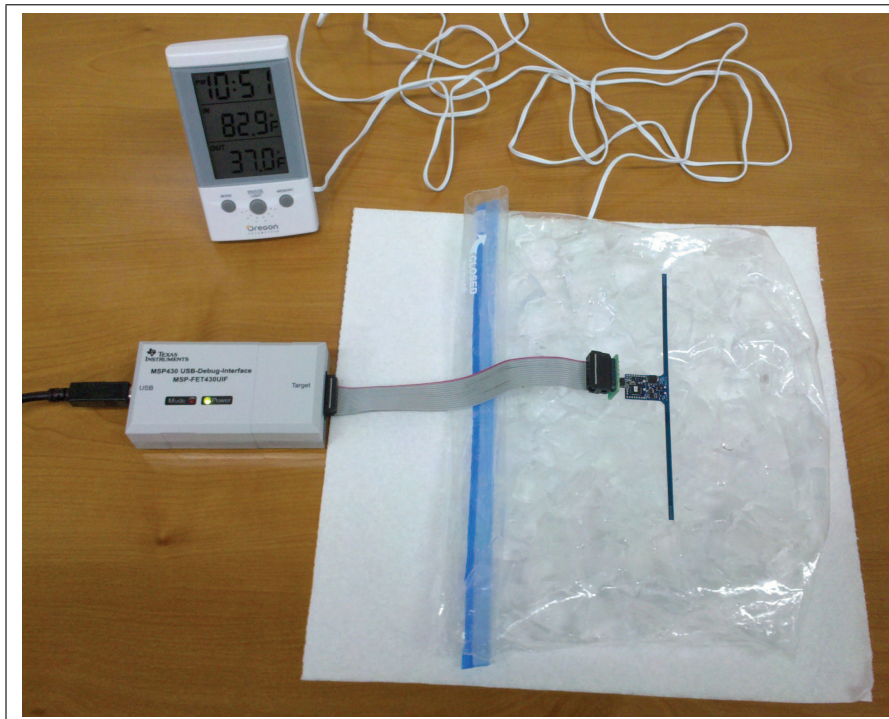
Fig. 4 WISP tag being cooled on a bag of ice while attached to MSP-FET430UIF debugging interface
