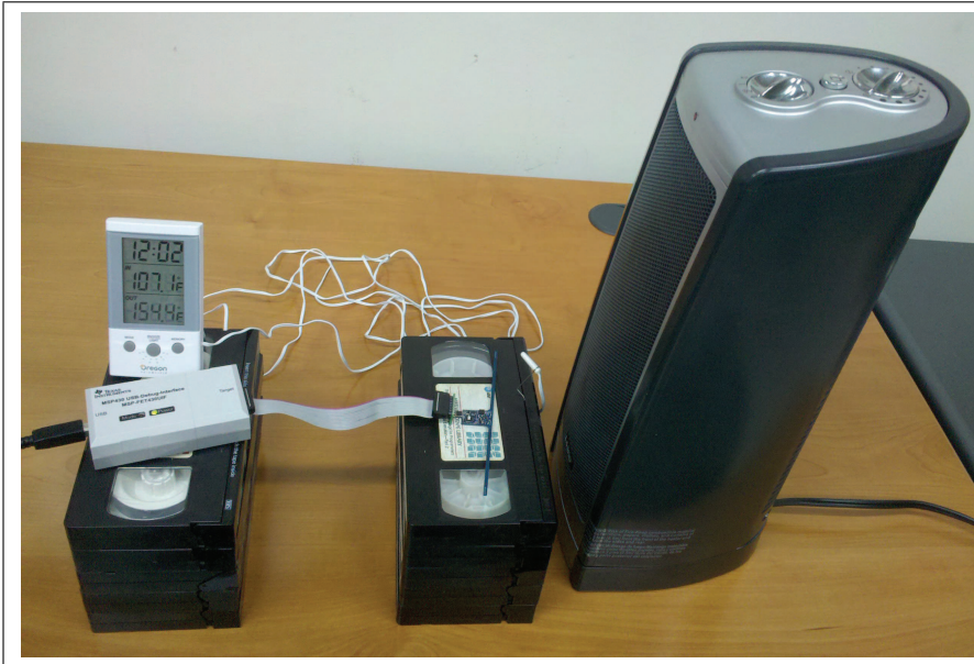
Fig. 5 WISP tag being warmed by an electric heater while attached to MSP-FET430UIF debugging interface
