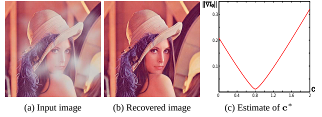
Figure 4: Simulation results for solving \mathbf{c} based on Equation (7). (a) A synthetic image with a dirty-lens artifact is generated using the lens dirt pattern extracted from Fig. 3(c). (b) Equation (7) is used to recover an artifact-free image, with a mean absolute percentage error of 0.44% compared to ground truth. (c) A plot of \|\nabla \mathbf{I}_0\|_1 versus \mathbf{c} . The optimal estimate, \mathbf{c}^* , has a 0.25% error compared to ground truth.
