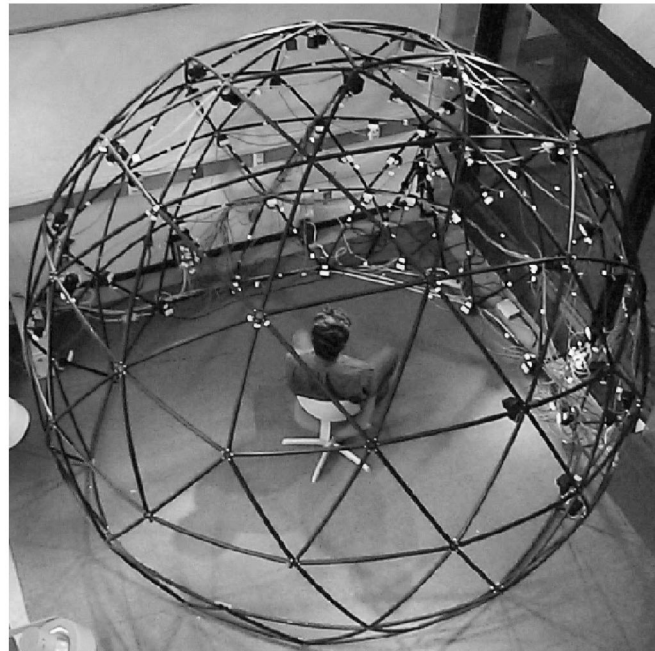
Fig. 10. A geodesic dome with 64 strobes used to gather images under variations in illumination and pose.
