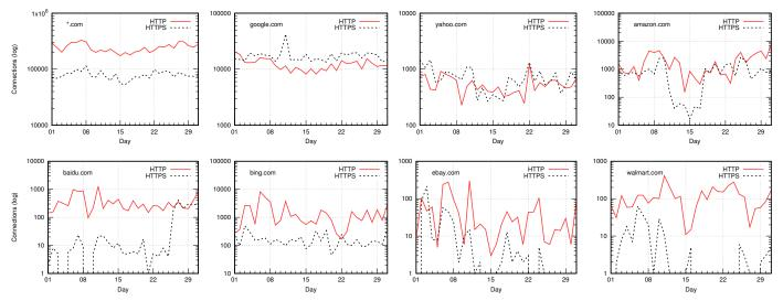
Fig. 5. Number of encrypted and unencrypted connections per day, as seen from a freshly-deployed Tor exit node.
