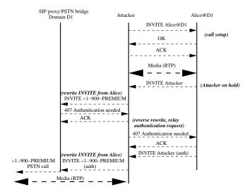
Fig. 5. SIP relay attack
