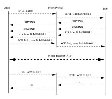
Fig. 2. Message exchanges during a SIP-based two-party call setup.
