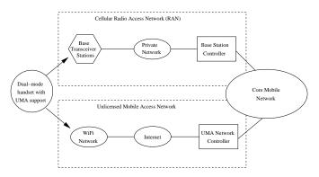
Fig. 4. Unlicensed Mobile Access (UMA) conceptual architecture
