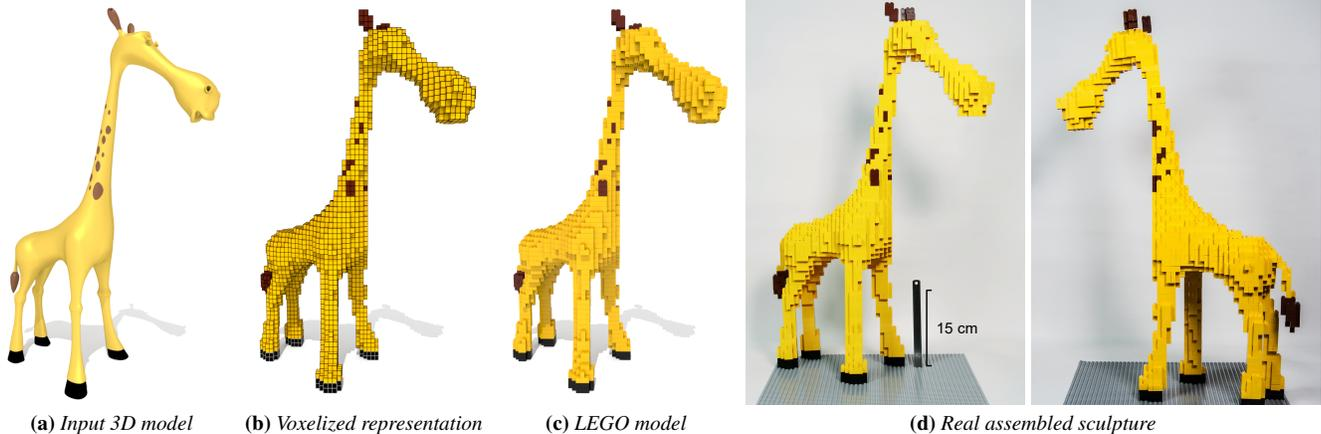
Figure 1: Our method transforms an input 3D model (a) into a physically stable LEGO model (c) that can be realized in the real world (d).
