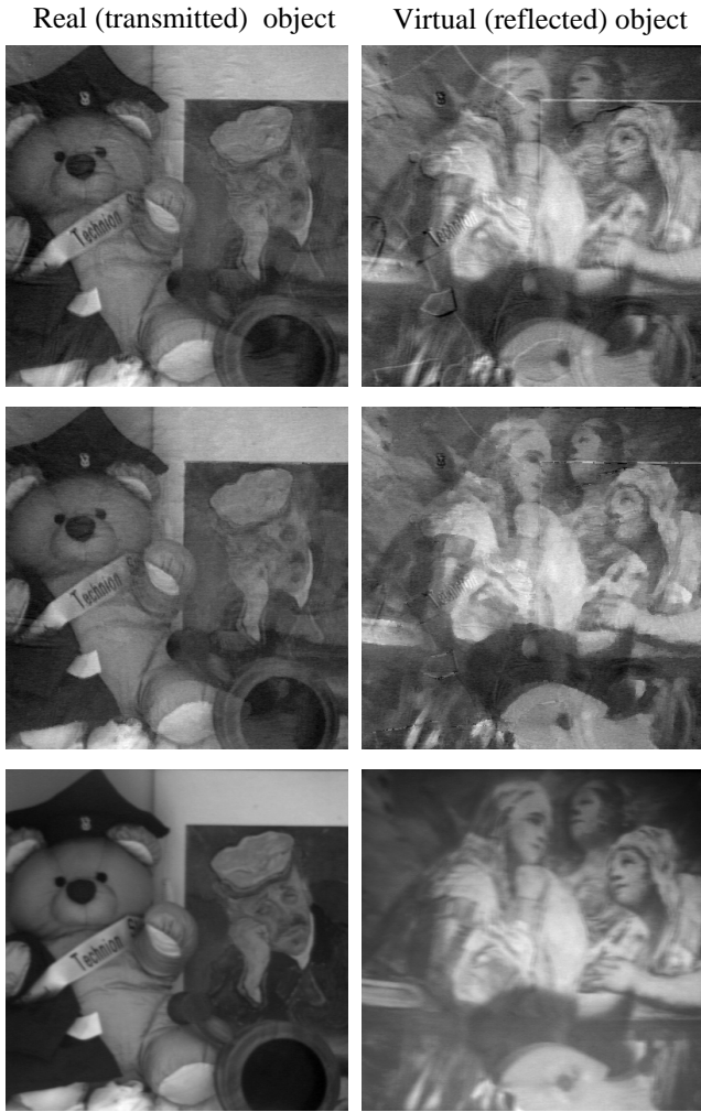
Figure 6: [Top row]: Reconstruction by pointwise operations. False edges are very disturbing in the virtual layer (as pointed out in Fig. 7). [Middle row]: Reconstruction using local shifting corrections. Most of the disturbing real-object edges disappeared from the reconstruction of the virtual object. [Bottom left]: The real object photographed without the interfering glass window. [Bottom right]: The virtual object photographed by removing the objects behind the glass window.
