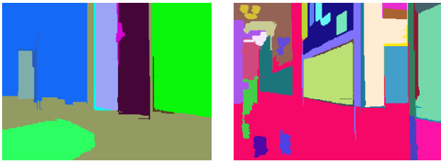
Fig. 7. The result of graph-based segmentation [5] on two corridor images used in Figure 6, with each region assigned a random color. Note that the floor is almost a homogeneous area in both images, while the wall and doors are divided into several smaller regions.
