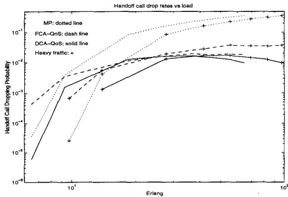
Fig. 9. Comparison of DCA-QoS to FCA-QoS and MP: Non-uniform Traffic. “—”: DCA-QoS; “- - -”: FCA-QoS; “...”: MP. Curves with “+”: Heavily-loaded; curves without “+”: Lightly-loaded.
