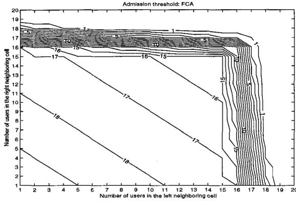
Fig. 5. Contour of Admission Threshold for the FCA-QoS ( $M=40$ ).
