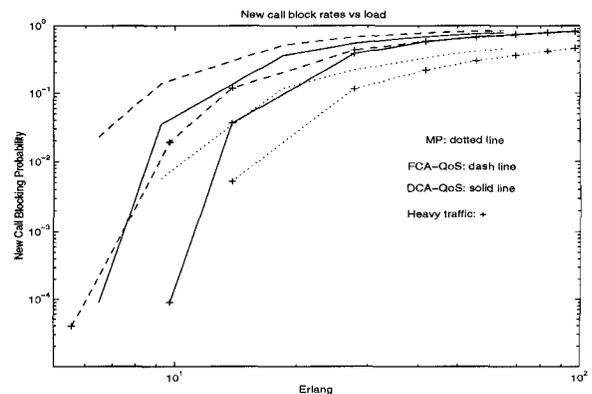
Fig. 8. Comparison of DCA-QoS to FCA-QoS and MP: Non-uniform Traffic. “—”: DCA-QoS; “- - -”: FCA-QoS; “...”: MP. Curves with “+”: Heavily-loaded; curves without “+”: Lightly-loaded.
