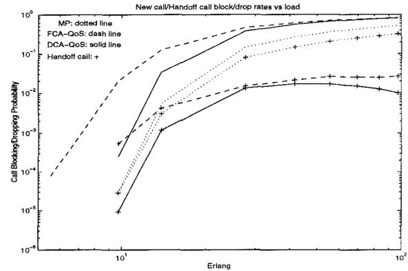
Fig. 7. Comparison of DCA-QoS to FCA-QoS and MP: Uniform Traffic. “—”: DCA-QoS; “- - -”: FCA-QoS; “...”: MP. Three curves from the top without “+”: new call blocking probability  $P_B$ . Three curves with “+”: hand-off dropping probability  $P_D$ .
