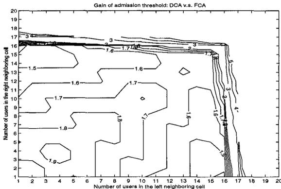
Fig. 6. Contour of Admission Threshold Gain for the DCA-QoS over the FCA-QoS ( $M=40$ ).
