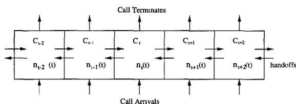
Fig. 1. 1-D Cell Array
