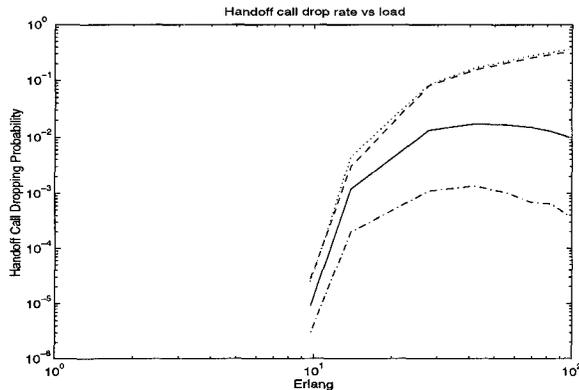
Fig. 2. Comparison of QoS Threshold ( $P_{DQoS} = 0.01$ ). “- · -”: FCA-QoS; “—”: DCA-QoS ( $P_{BQoS} = 0.2$ ); “- - -”: DCA-QoS ( $P_{BQoS} = 1.0$ ); “...”: MP.
