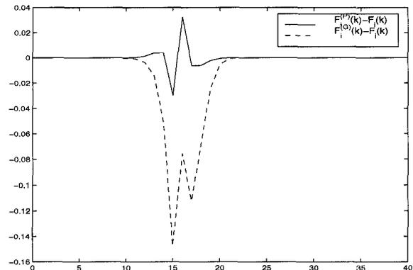
Fig. 4. Approximation Error to  $F_i(k)$  ( $M = 40$ ,  $N_i(t_0) = 16$ ). “—”:  $F_i^{(P)}(k) - F_i(k)$ ; “- - -”:  $F_i^{(G)}(k) - F_i(k)$ .
