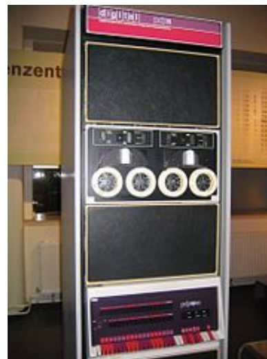
A PDP-11, model 40, an early member of DEC's 16-bit minicomputer family, on display at the Vienna Technical Museum
