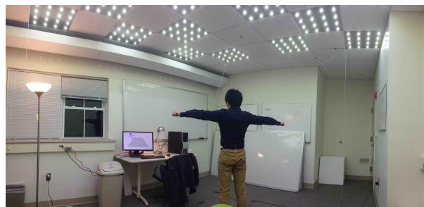
Figure 1: StarLight reuses ceiling LED panels together with a few photodiodes to reconstruct a mobile user’s skeleton in a normal office setting with furniture.
