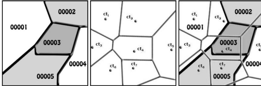
**Fig. 2.** (Left) Example of Geographical Regions (GR) that have a SEL associated; (Center) The same geographical areas with the BTS towers (coverage approximated with Voronoi tessellation) and (Right) The correspondence between GRs and BTS towers used by a scanning algorithm to assign a SEL to a BTS tower area.
