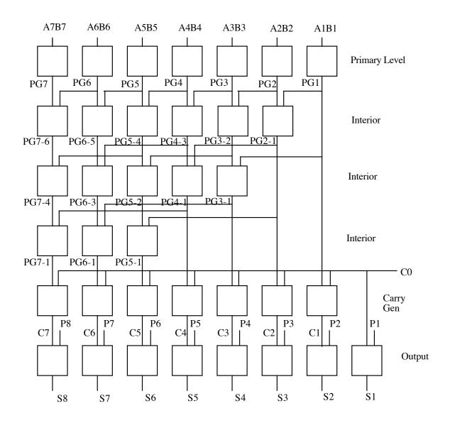
The primary level modules produce the G and P signals corresponding to the input pairs. The logic is:  $Pi=Ai\Theta Bi$ , Gi=AiBi.
