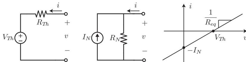
**Figure 3:** The  $i$ - $v$  characteristic of the equivalent circuits
