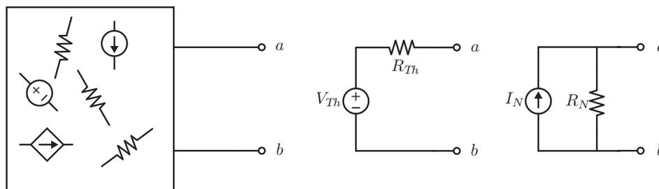
**Figure 2:** The Thévenin and Norton equivalent circuits
