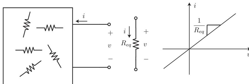
**Figure 1:** A “black box” of resistors, its equivalent resistance, and their  $i$ - $v$  characteristic
