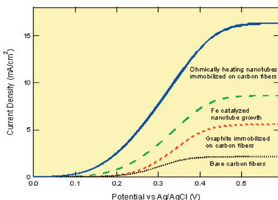
Figure 4. Polarization of the glucose oxidase anode from different support morphologies. Experiment conducted under N<sub>2</sub> in pH 7.1 PBS buffer at 37.5°C, 50 mM glucose, on a rotating disk electrode at 4000 rpm rotation rate. Current densities were based on the area of the 4-mm carbon cloth disk (0.13 cm<sup>2</sup>), and 39.6 wt% GOx (with NaIO<sub>3</sub>), 59.5 wt% PVP([Os-bipy]<sub>2</sub>Cl), 0.9 wt% PEGDGE at 0.32 mg/cm<sup>2</sup> GOx loading.
