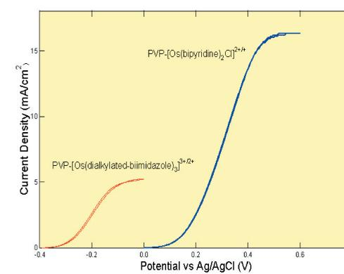
Figure 7. Polarization of the anode supported by Ohmically-heated carbon fiber, mediated by different redox species. Other conditions as in Fig. 4.
