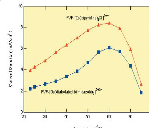
Figure 8. Temperature dependence of maximum current density on 190  $\mu\text{m}$  nanotube-treated carbon paper. Electrodes poised at 0.5 V vs Ag/AgCl for PVP([Os-bipy]<sub>2</sub>Cl), 0.0 V vs Ag/AgCl for PVP[Os(da-biimidazole)<sub>3</sub>]. Other conditions as in Fig. 4.
