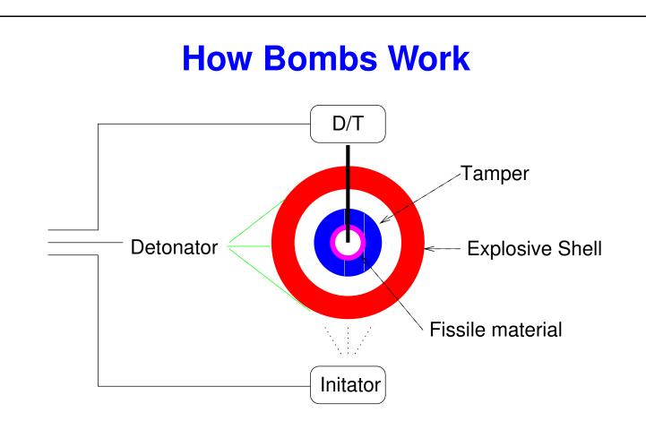
The deuterium/tritium pump, the initiator (the initial neutron source), and the detonators are all controlled by the sequencer. The first two require high voltage sources. Timing is critical to yield.
