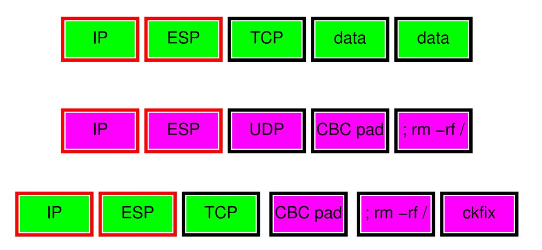
Use the target's TCP header, plus attack text encrypted for the enemy. Calculating a checksum fix-up isn't hard, and is only 2<sup>16</sup> tries anyway
