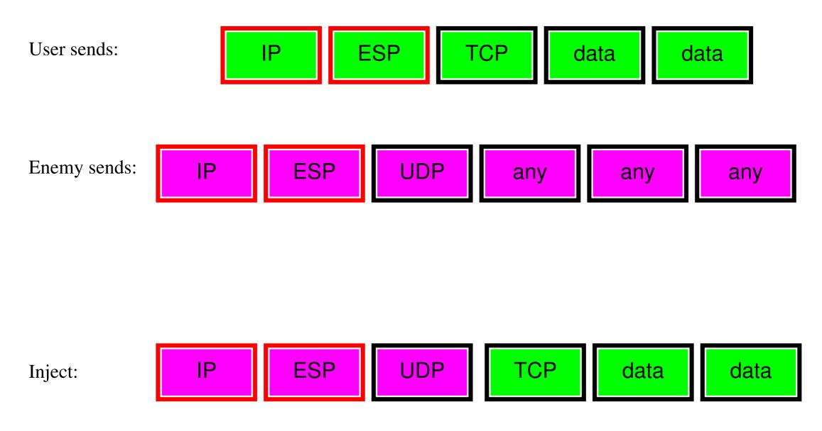
Paste together enemy UDP header with target's payload – and IPsec will do the decryption for the attacker
